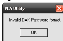
Figure 29 Incorrect DAK or No DAK
